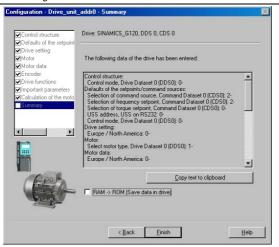
To complete basic commissioning, the motor data identification, selected during basic commissioning must be performed via switching on the inverter. This can be done via the chosen command source (e.g. terminals, BOP or communication) or via STARTER as shown in the dialog box below.
