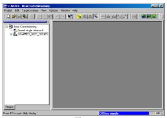
To go online with this inverter press  $\[ \frac{\mathbf{Q}_{m}}{\mathbf{Q}} \]$ . The following dialog box shows in the left column the online and in the right column the offline saved data. To load the online data to your PC, press "Load HW configuration to PG" and end the dialog with close.
