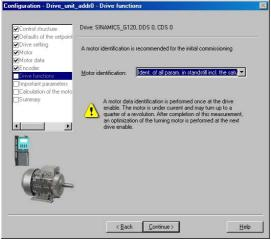
For calculation of the motor data we recommend to select "Restore factory setting and calculate motor data only" as shown in the dialog box.
