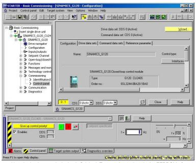
Now the basic commissioning is finished. To save the settings in the EEPROM of your inverter, select the SINAMICS project and press the "Copy RAM to ROM" button ...
