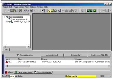
It states that no commissioning has been performed so far with the inverter. To confirm, select the message and press the "Acknowledge" button.
